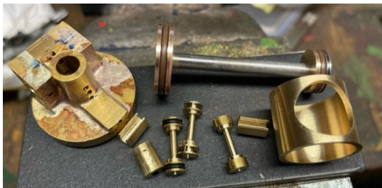
Spare shuffles and valves were made.
