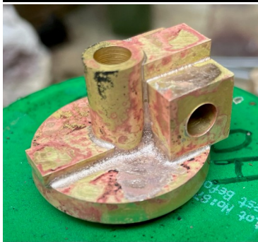
The first step. The five piece head was silver soldered.
