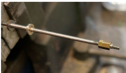
The trip rod, with pilot valve cradle and trip button nut and lock
