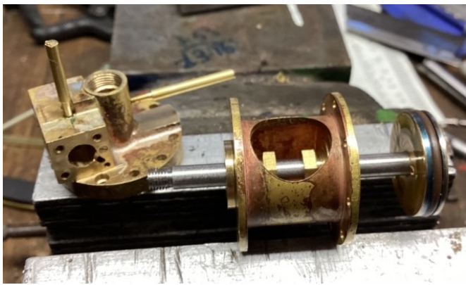
Plugs of 8 and 9 BA were made by Loctiting in a few turns of thread and later Dremeling off flush, and reusing the threaded rod end in the next session.
