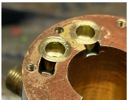
Mistake on mistake. Wells inserted to remake the ball seats.
